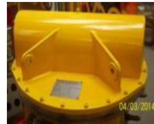
SCM ready for installation
