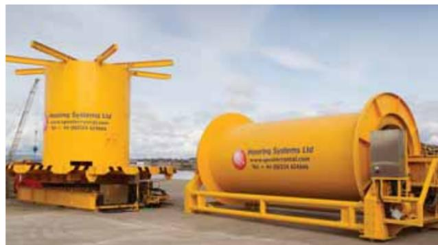
Offshore handling equipment specialist, Caley Ocean Systems Ltd, has designed and built what is believed to be the most adaptable offshore, mobile turntable of its kind in the UK, for spooling equipment hire company Mooring Systems Ltd in Aberdeen. Capable of handling a wide range of flexible products including cables, umbilicals, dynamic risers and hoses, the 400 tonne modular turntable spooler can be readily configured in either 'reel' or 'basket' modes; and is both sea and road transportable.
