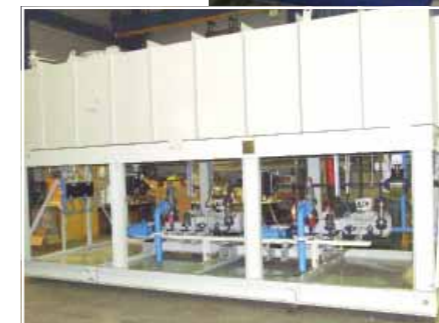
Left: Litre Meter has supplied VFF meters to Geveke Pompen used to monitor MEG which helps prevent hydrate formation in lines on the new Wingate natural gas well in the North Sea
