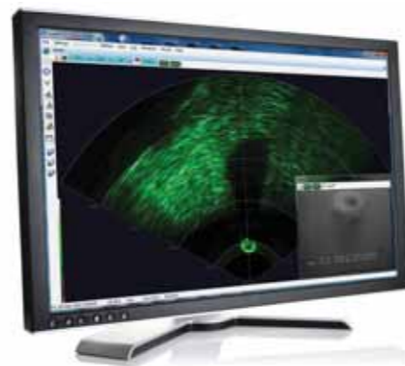
Seanet Pro windowed layout showing Gemini 720i sonar image of a sunken barrel
