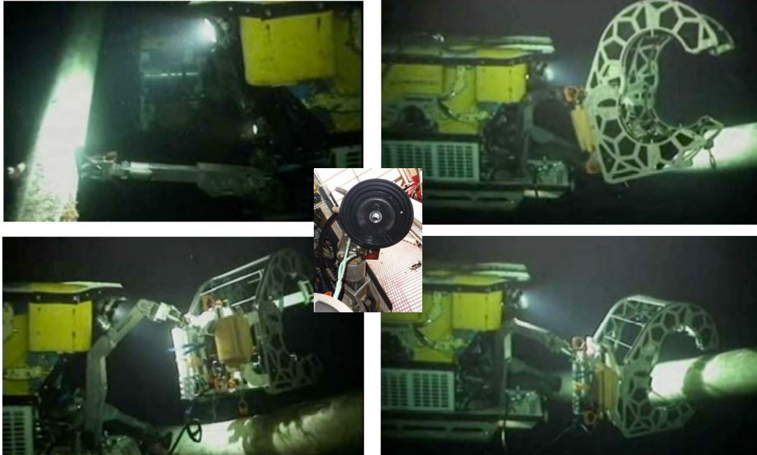
Work Class ROV deployment – using 'sticky foot'
