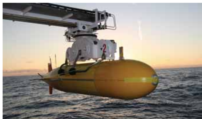
Autosub6000: Final checks before launch on its first ever deep mission to 4553m depth.
